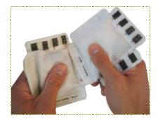
Lightweight foam padding inside each module provides cushioning against the electronics. For the outside of a bYOB block, a simple nylon fabric was chosen because it is a tolerant material with the ability to act as a fabric interface and dissipate light from any LEDS embedded within.
