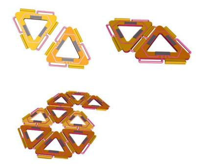
Printing this connector technology out on the FDM (fused deposition modeling) machine revealed that neighboring connections were loose. Moreover, because a separate channel for electrical conduction would have to be added into the design, the method proved too complex to pursue any further.
