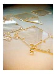
Commercial metal snap connectors acquired from a fabric store seemed to circumvent these problems because of their unambiguous, secure design and their clear performance as conductors. 3.1.8 commercial snap metal connectors found to be secure, and conductive
