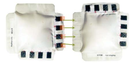
3.3.3 GND, SDA, SCL, PWR hook and loop pads As stated before, corresponding pads on each edge are connected together via internal wiring so the ground pad on one edge is connected to all of the corresponding ground pads on each subsequent edge- and so on for each type of pad.
