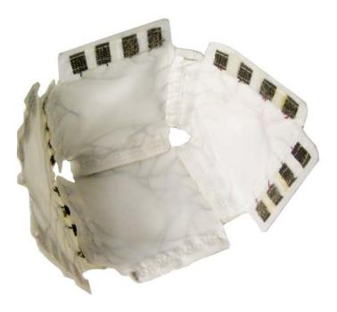
The front and back of a block actually corresponds to an inside or an outside of a fabric object. It is easy to tell what side is an outside because it is adorned with non-conductive Velcro used to "skin" any object built out of the system with decorative fabric. Because of this feature, the system aesthetic is also modifiable.
