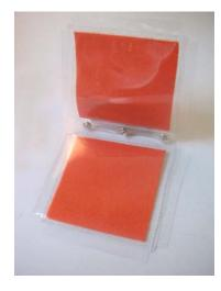
It was decided early on (for reasons that will be explained later) that the communication bus would be a four-channel protocol that transmits power, ground, data, and clock through the conductive snaps. A diagram indicating how the printed circuit board (PCB) could be wired to the snaps was mocked up and construction on the blocks began.
