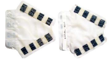
To connect two blocks together, a user simply ensures that both sides of a block are facing the same direction in or out, and then their corresponding hook and loop pads align.
