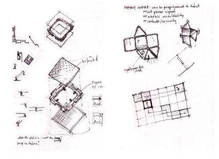
Simple geometries of squares and triangles were chosen because they are easily recognizable and can be effortlessly manipulated into two and threedimensional shapes. Additionally, the dimensions were chosen to fit comfortably when grasped by the human hand. Next, modular shape choice and its influence on an object's degree of configurability were investigated. 3.1.2 2d study of triangle and square geometry configuration
