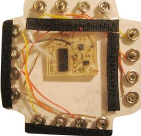
Tangible study revealed that the snaps were ultimately disappointing because their aggregate weight compromised the feel of any object that was constructed out of such a configuration.
